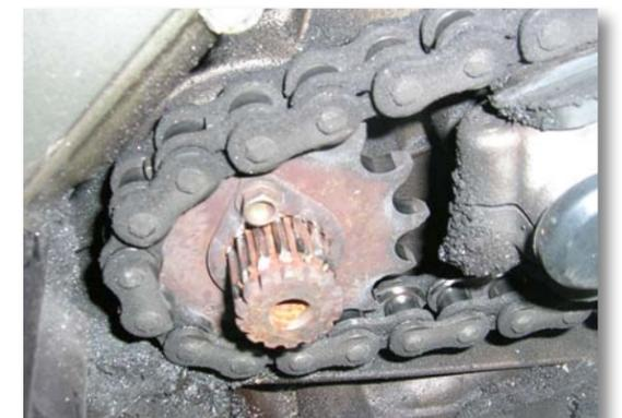
Showing how badly the sprocket has drifted toward the engine case
