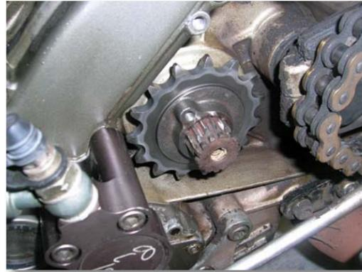
Worn sprocket pushed as close to the case as possible
