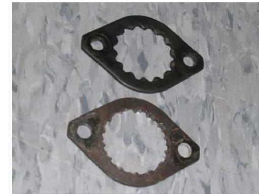
Showing the difference between the worn retainer and a new one
