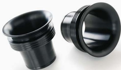
The Ducshop Hyper Stacks eliminate the stock airbox on the dual-spark motors, replacing it with two stacks and individual pod filters, giving double the air filter surface area over stock filters. The entire kit cost just \$275 and includes stacks, K&N pod filters, crankcase filters and idle filters and boasts a six to eight horsepower increase.
