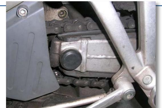
The misaligned chain with the chain guide on the swingarm
