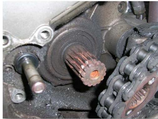
Shows the wear on the inside of the tranny output shaft splines
