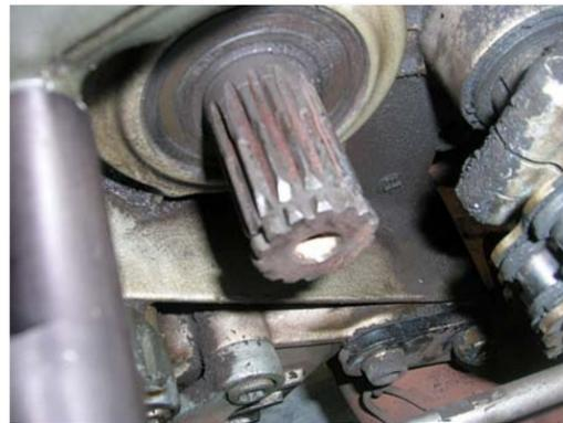
Spline wear after the second failure
