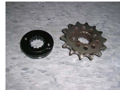
The modified sprocket/spacer and a sprocket for comparison
