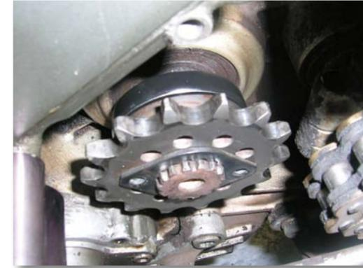
Spacer, sprocket, and new retainer test fit on the output shaft
