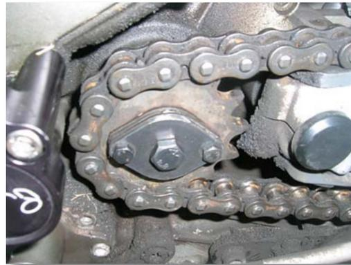
Failed attempt at using the end of the output shaft to hold the sprocket in place
