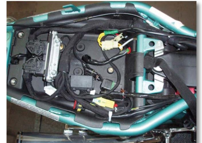
First try top view with wire routing. Notice the brass capture nuts that have the regulator bolts coming up from the bottom.
