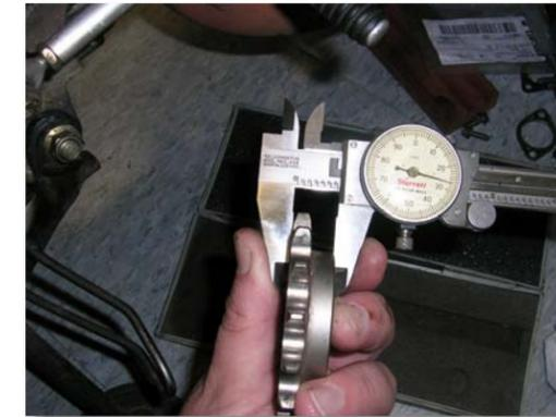
Measuring the width of the sprocket
