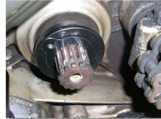
Spacer on the output shaft
