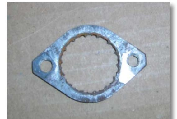
Shows the teeth on the sprocket retainer worn to a point
