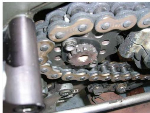
Sprocket drift from the second retainer failure
