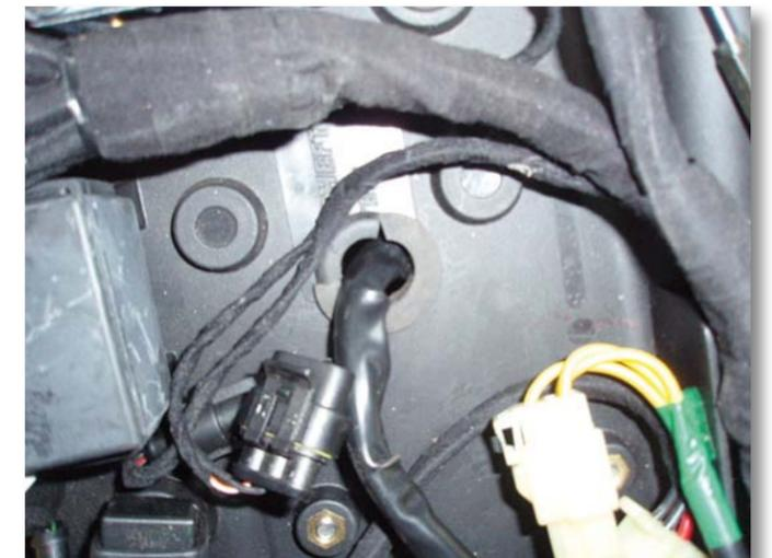
Grommet has now been added to protect the wiring. Those of you with sharp eyes will note I need to find a bigger grommet.
