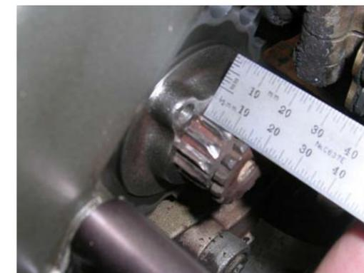
Measuring the distance between the worn sprocket and the inside of the retainer groove
